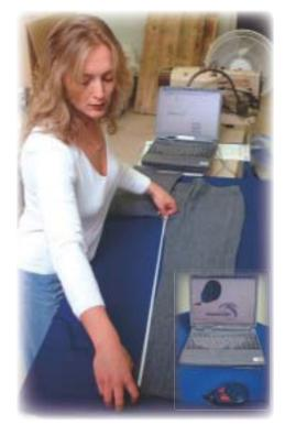
The Dimension Link tape measure brings accuracy and objectivity to measurements on the shop floor. Designed for use in a factory and retail environment, the tape handles like an ordinary cloth tape measure, but records dimensions directly onto a computer screen.
